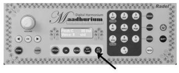
**11.3.3** On completion of tuning as above, press OK to exit the Key Tuning Mode.
