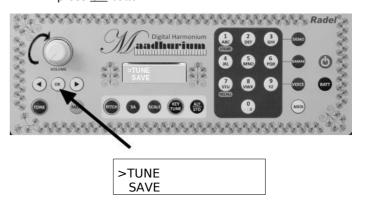
**11.3.2** Press the note key to be tuned. For manual tuning, turn the knob for raising or lowering its pitch as desired. For 22 Sruthi tuning, press ALT/STD for selection of one of the two settings for that key.
