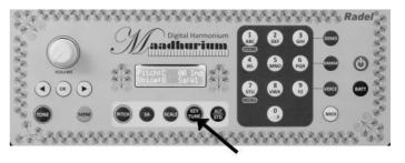
**11.3.1** TUNE/ SAVE/ RECALL option is displayed on LCD. Within 4 sec, select TUNE using knob and press OK button.
